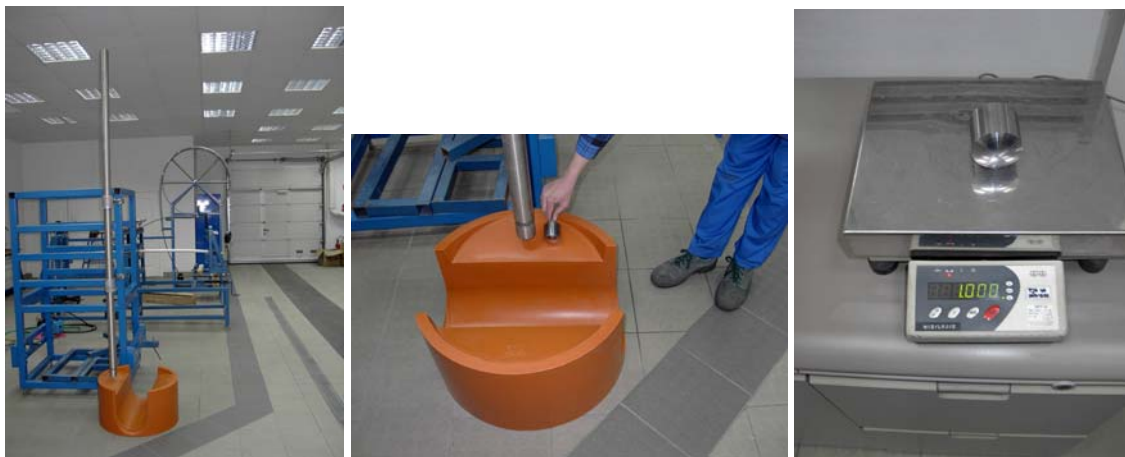
Figure 1B: Impact test set up for the rotational moulded shells. The left picture shows the full set up, the middle picture shows the alignment at the place of impact and the right picture shows the used impact weight.
