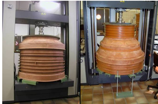
Figure 4A: Testing of the 800 cone on a 800 riser
