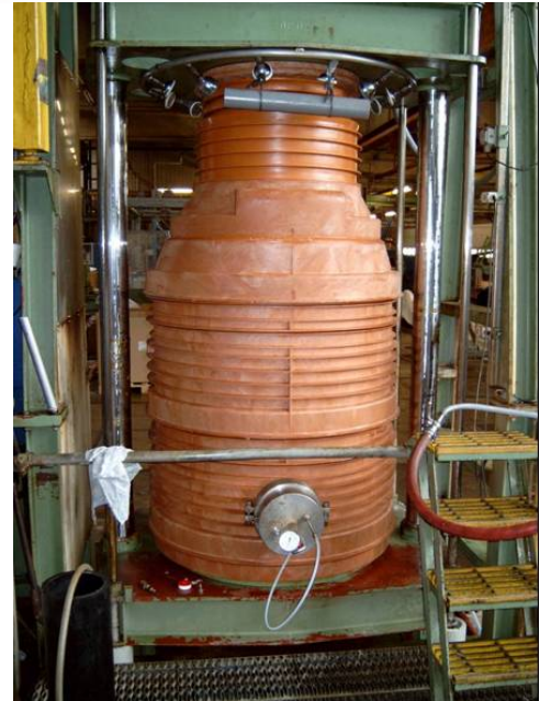
Figure 2: Test set up for internal pressure test
