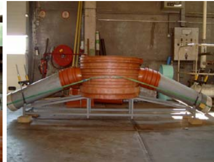
Figure 3B: Test set up for mechanical testing of the fittings and inlet/outlet adapter under the angle of 25° (left and right) on PRO1000 manhole.
