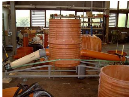
Figure 3A: Test set up for mechanical testing of the fittings and inlet/outlet adapters under the angle of 25° (left) and 10° (right) on PRO800 manhole.
